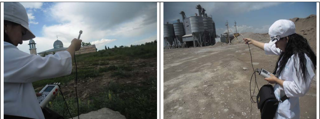
Noise and Vibration Monitoring near mosque at turning of Crushing Plant (left) and at Concrete batch Plant (right)
